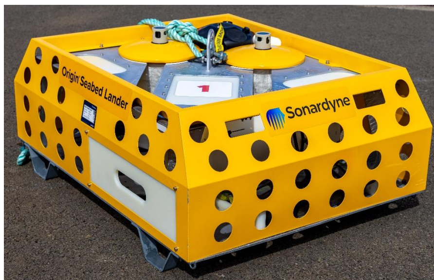
Figure 2: Photograph of lander bedframes to be deployed at locations marked by yellow squares. Bedframes will be deployed as standalone units without surface markers or ground lines. Recovery will be handled by activation of acoustic releases which will deploy a buoy from the bedframe carrying a recovery rope to the surface. Each lander bedframe has two of these buoys to provide redundancy
