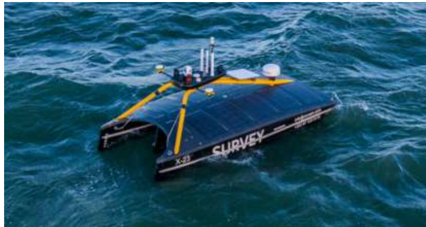
Figure 2: USV with hull mounted sensors
