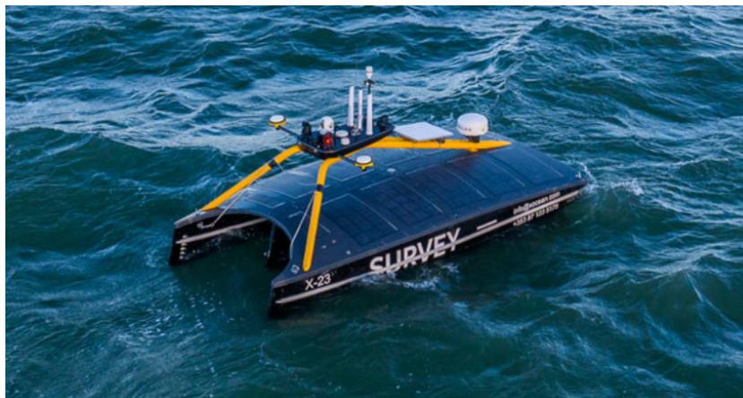
Figure 2: USV with hull mounted sensors
