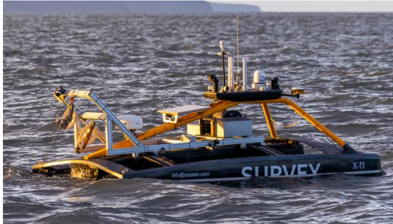
Figure 3: USV with towed sensors
